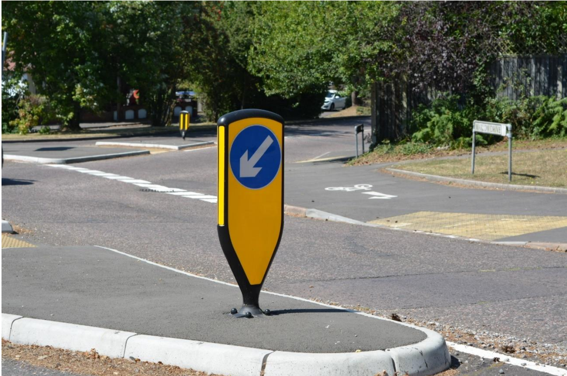
Figure 6: Example of Retroreflective self-righting bollard (RSRB)
